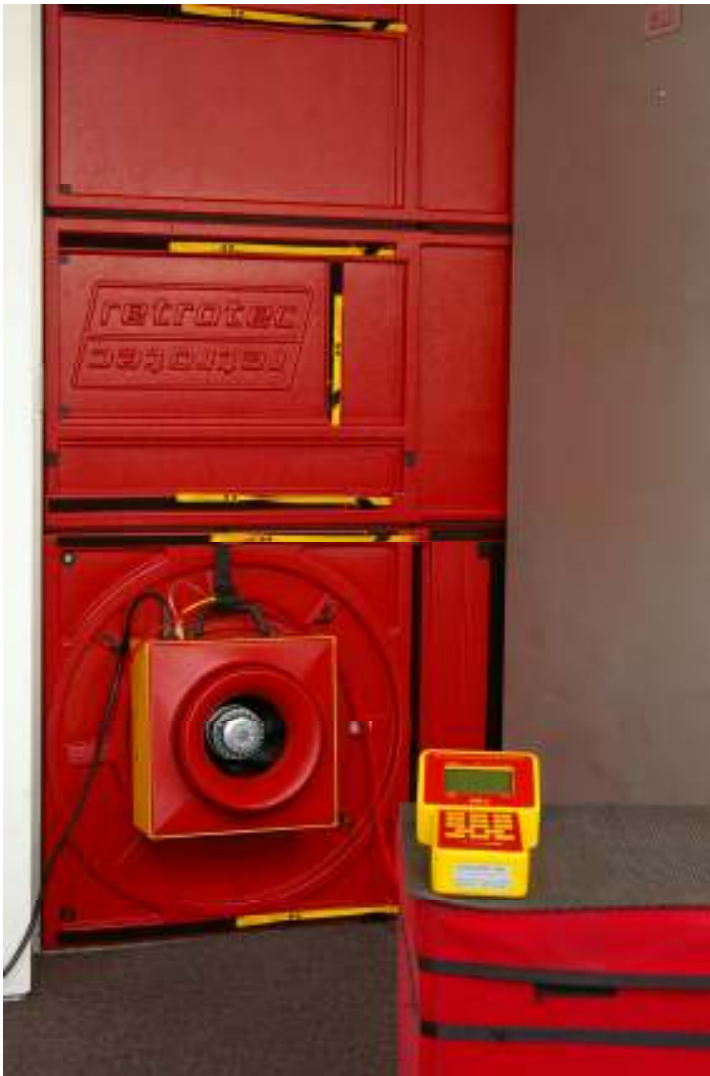
Retrotec Model Q52 consists of a DM-2A, a DU-220 Low Flow Fan and Single Fan Modular Panel Set-Up.
